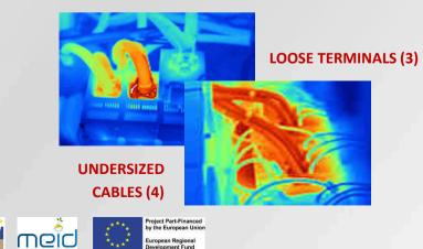
These pictures show others thermographic measurements but, in this case, we can see industrial equipement. Especially in the existing plant systems we can found conditions such as those represented in the images. Inefficiencies due to damaged insulation or insulation evil placed, incorrectly connected terminals or undersized cables.
