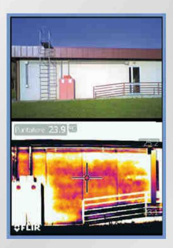
If we observe the images we see that there are high heat loss and this is an indicator that communicates the absence of insulation on the perimeter walls. It is needless remembering that to an increasing heat loss corresponds an increase of the fuel that we canto burn to maintain a good temperature inside and thus it increase the emissions into the atmosphere.
